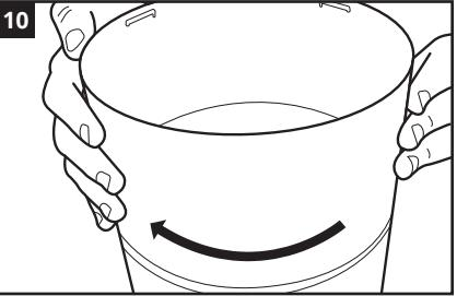
**EN** Rotate the reservoir clockwise until it locks into place.
